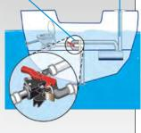
■ Type III MSDs, the simplest and most common, consist of holding tanks or portable toilets. Waste is to be taken ashore and disposed of in a pump-out facility station.
